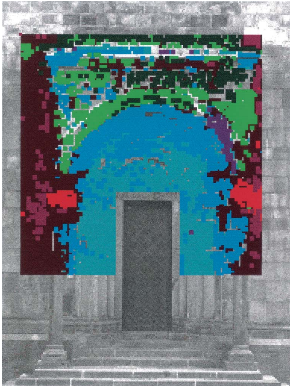
Fig. 10. False-colored image with pixels superimposed upon a photograph of the northern portal. Areas with different characteristics can be identified. Thus, pixels with 12th-century stone characteristics are shown in blue-indigo, and those with 19th-century characteristics are shown in green. The violet pixels correspond to areas that exhibit iron-ion quenching. The normalized chlorophyll pixels from Fig. 8 have been merged in red color tones: Pixels with a large amount of biodeteriogen PC1 are light red; those with a high PC2 score, darker red; and those with both PC1 and PC2 low are shown in a very dark red color.
