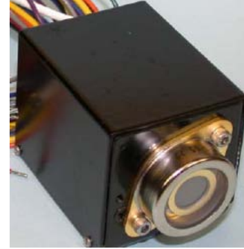
Figure 5.13. View of a red enhanced silicon large area ( \phi=10 mm) APD module (SD394-70-72-661, Advanced Photonix).
