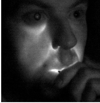
Figure 2.6. A measurement of light scattered in a human head and sinuses by the use of a IR-LED (LED760/940-04A, Roithner Lasertechnik) and a IR-CCD camera (C5999, Hamamatsu). The light source is mounted in a similar position as explained in Paper XII.
