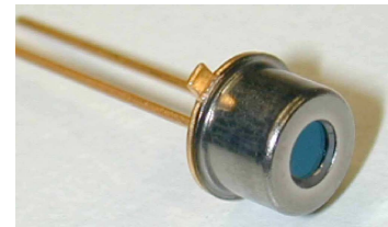
Figure 4.8. A VCSEL laser in a standard TO 46 can without a build-in Peltier cooler; from [56].
